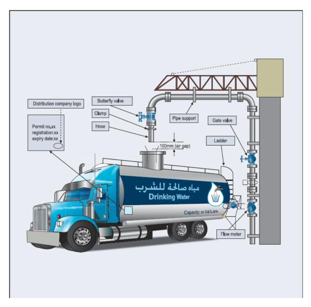
The above diagram is for illustration purposes only. All potable water tankers must comply with the relevant clauses of the Water Supply, Tankering and Water Quality Regulations, in addition to the Distribution Company's own requirements.
