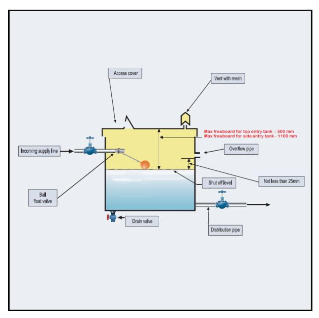
The above drawing is for illustration purposes only. General requirements for tank connection, fittings and accessories are dependent on the tank location, volume, height and material of construction as prescribed in this Guide. However, the standard requirements for a tank are that it should be provided with a flow-control device (float-operated valve), an overflow pipe, access/ an access cover, service valves, a vent and drain connection (as necessary).
