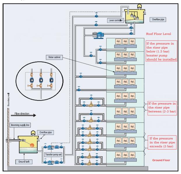
D.6 - Typical internal connection arrangement for a high-rise building (metered internally).
