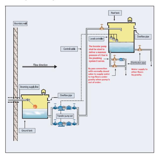
D.4 - Typical connection arrangements between ground and roof tank in low-rise and high-rise buildings.
