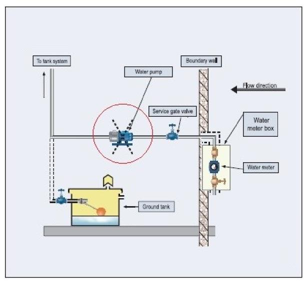
D.8 - Prohibited connection arrangement: the installation of an on-line pump that draws water directly or indirectly from the main distribution pipeline.
