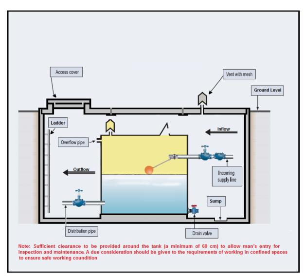
The above diagram is for illustration purposes only. Underground tanks are only permitted in basements or in purpose built underground pump rooms upon approval of the Distirbuation Company.
