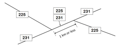
Figure 7: Connection Between Two Routes Less Than 1 KM
