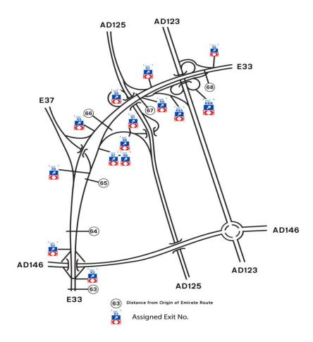
Figure 12: Illustration of Exit Numbering
