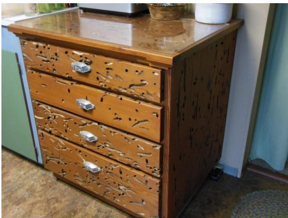
Dry wood damage on kitchen wooden drawers
