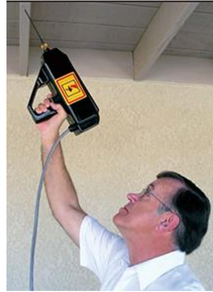
Dry wood electrocution treatment using electrogun
