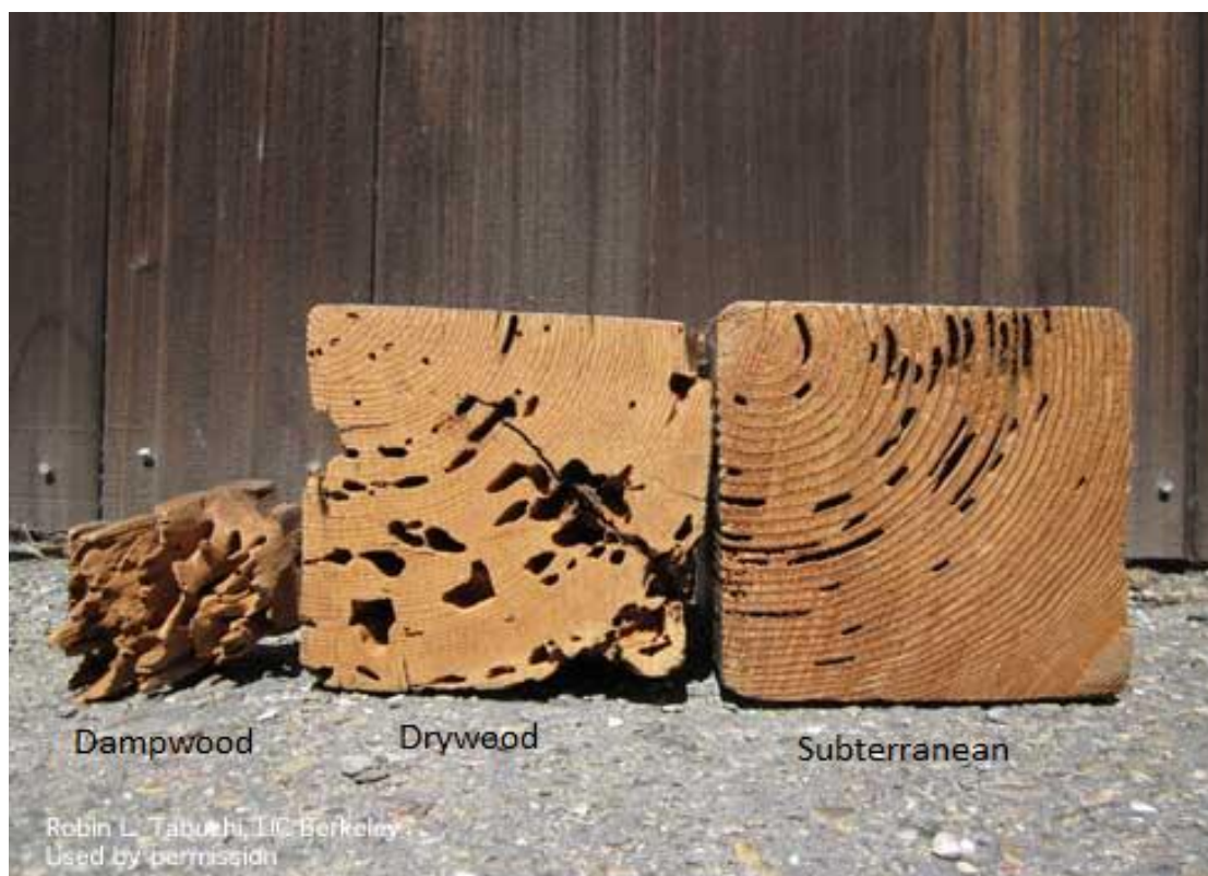
A Comparison between the damage of drywood, dampwood, and Subterranean termite
