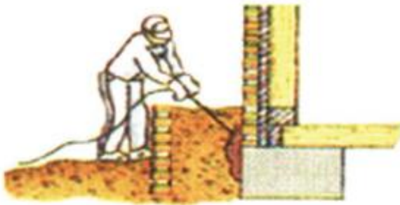
Use rod injection to treat soil along and around the external perimeter area of the building.
